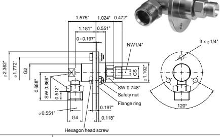
Throughput Medium: water, oil, compressed air pH 3-12
