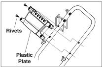
**STEP 4:** Attach the plastic plate from the top aligned to the four holes placed on top of the handle and insert the rivets through holes of plastic plate.
