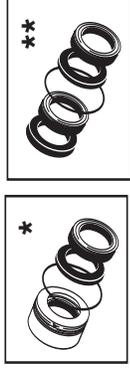
\* Plunger seal kit when the low pressure packing is preloaded into the cup retainer.
