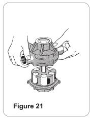
NOTE: If the End Plate has been resurfaced the Body face must also be resurfaced to allow for material taken off the End Plate. Follow same procedure as above with emery cloth. Before new parts are installed all burrs should be removed – particularly in the Rotor Slots and Body.
