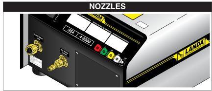
The five color-coded quick connect nozzles provide a wide array of spray widths from 0° to 45° and are easily accessible when placed in the convenient rubber nozzle holder, which is provided on the front of the machine.
